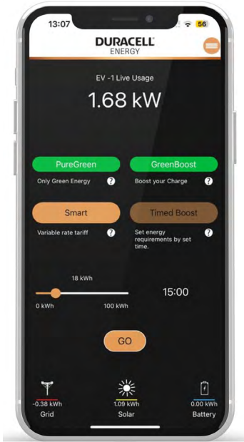
To change charging session mode whilst in another mode: Deselect current mode(s) Select desired new mode(s) Press 'Go'
